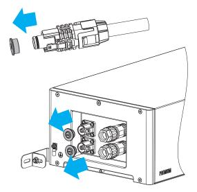
11. Plug the cables into the PDU. The other side of the cables should be well protected if it is not installed at this step.
