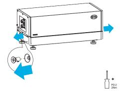
3. Put the installed base and feet along the wall, and keep the distance of 12~19 mm between the wall and the base.
