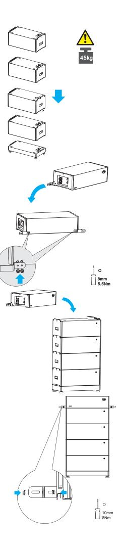
Fix the two hangers (wall part and PDU part) with M6X16 bolts and nuts, using a cylinder screwdriver (10 mm) to tighten it (torque: 8 Nm).
