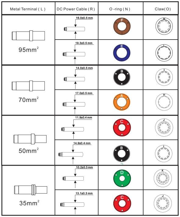
2. Install rubber core, O-Ring and cap in sequence on the DC cable.
